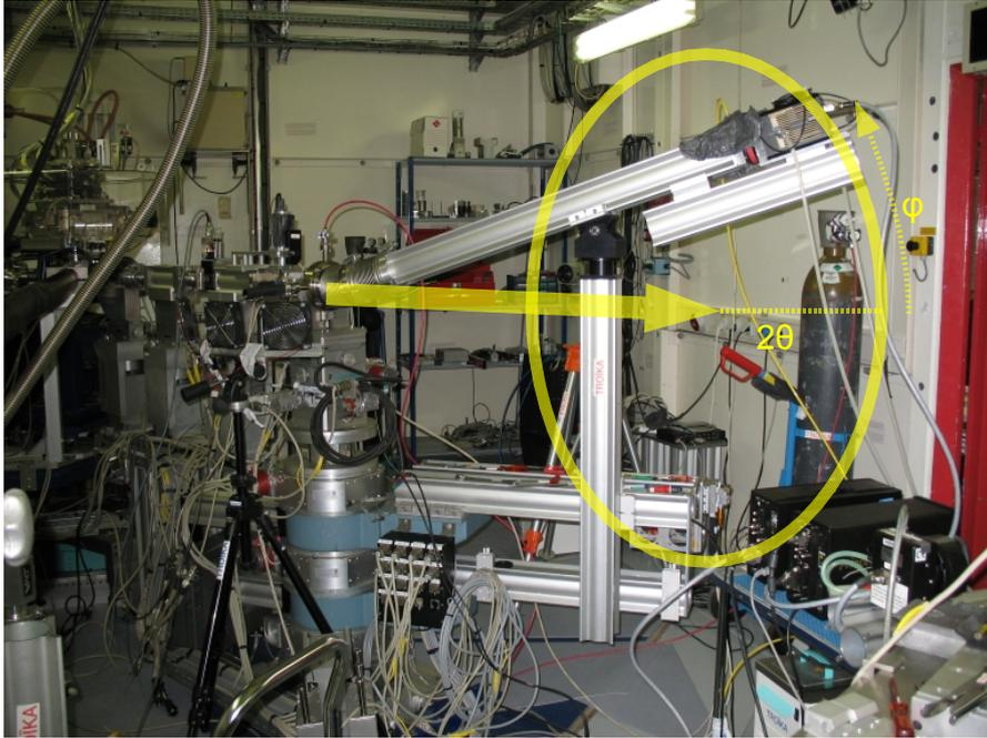
Figure A.2.: The set-up with the old furnace connected to the flight tube. Also visible is the PI CCD.
