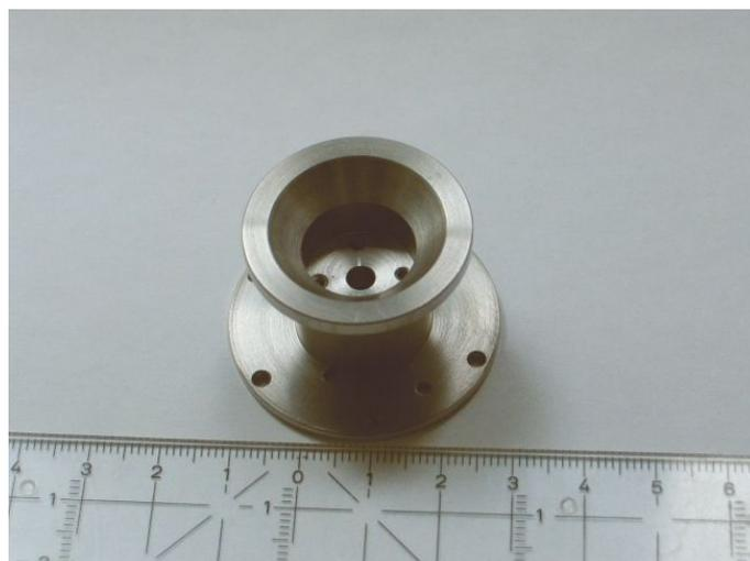
Figure A.1.: The heart of the old furnace. The sample holder is mounted inside, the heating wire is coiled outside.
